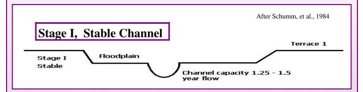
Stage I channel is a stable, relatively small channel that carries water and sediment in a manner such that the stream is neither aggrading or degrading. This does not mean that Stage I streams do not change positions in the landscape. Even though a stream is considered stable, it still has the ability to adjust, and is considered to be in a state of DYNAMIC EQUILIBRIUM.
