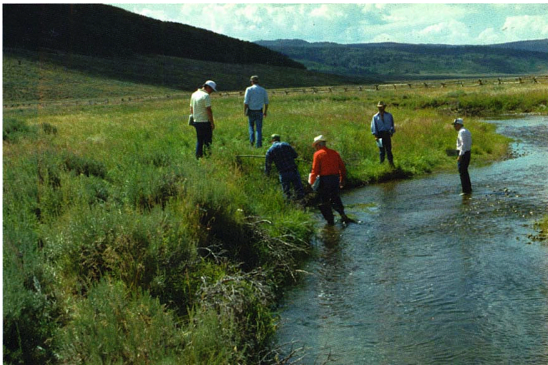
Figure 15 —Samplers using a 6-foot pole to measure woody species regeneration along the greenline.
