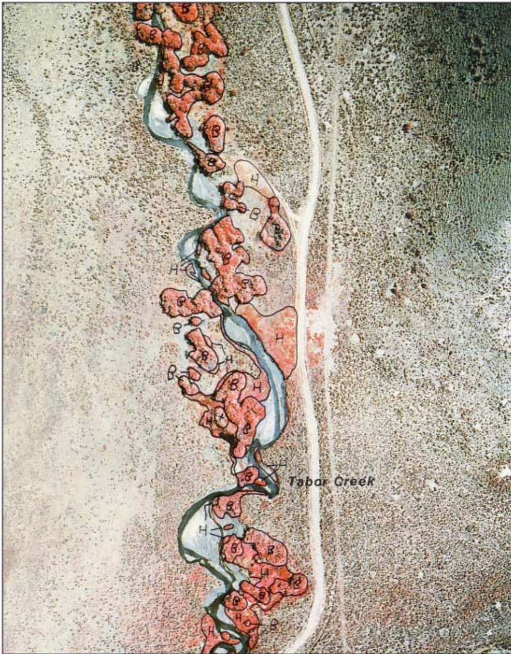
Photo 7 is a portion of a color infrared aerial photo of Tabor Creek, Nevada, acquired July 16, 1984, at approximately 1:2,400 scale (i.e., 1 inch represents 200 feet). Interpretations were compiled on clear mylar overlays registered to the fiducial marks on the photo.
