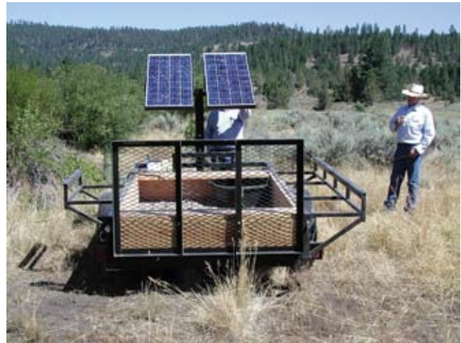
Figure 20. Mobile solar powered pump.
