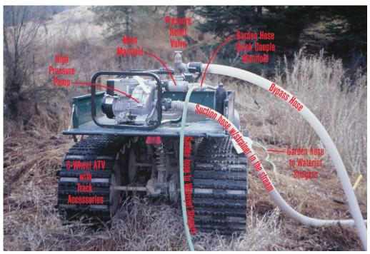
Figure C17-6-wheel ATV with track accessory
