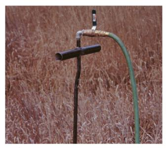
Figure C4-Handle with ball valve.
