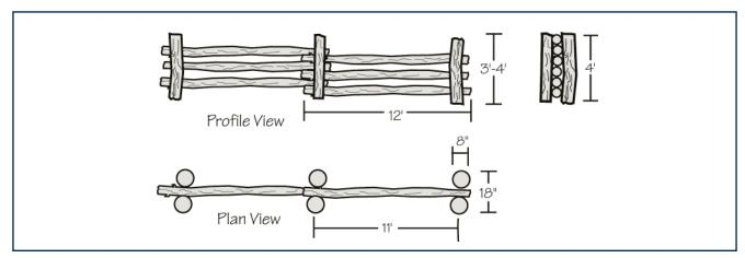
Figure E2-Double post with stacked-rail fence.
