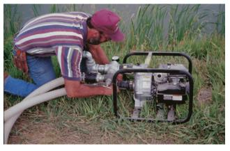
Figure C15-Note: Metal cage around the pump and motor was purchased separately.
