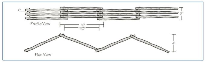
Figure E4-Parallel zigzag fence.
