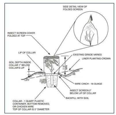
Figure D4-Liner planting with planter and screen
