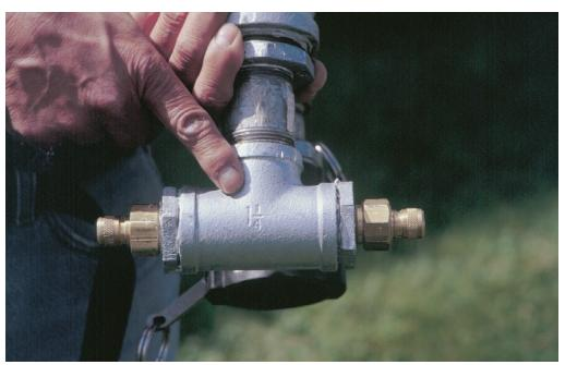
Figure C14-Garden hose quick coupler manifold.
