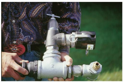
Figure C13–Waterjet Stinger manifold.
