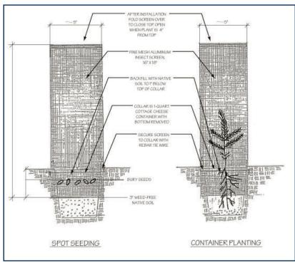
Figure D3-Collar and screen method
