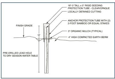
Figure D2-Plant tubes
